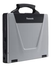
Left desperate, I bought her a late 2007, second-hand, semi-rugged Panasonic Toughbook™ CF-52 Mk1. This ageless, MIL-STD-810F standard notebook features an Intel® Core™2 Duo Processor T7100 —2MB cache, 1.80GHz clock speed, 800MHz FSB—, 2048MB 667MHz-clocked DDR2 RAM, Intel® GMA X3100 graphics and of course a carrying handle. It weighs in at 3.45kg without counting its sizeable 0.82kg, 8A, 15.6V power "brick". Not that this computer consumes a lot of power; the high current rating is for
